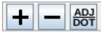
Figure 2. The buttons for importing assemblies. These commands are also available in the File menu.
